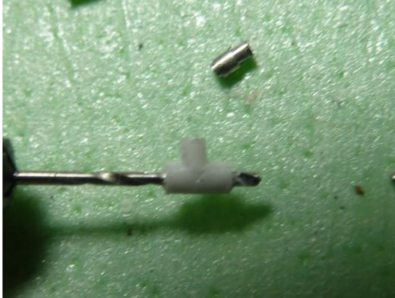
Making a Air Line T Pipe from .040 styrene rod Drilling a .020 hole for air line
