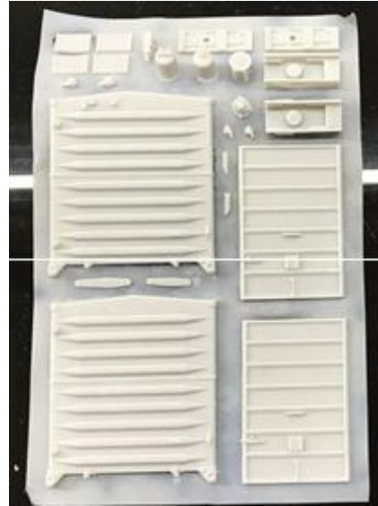
HO Scale Resin Parts showing PS Carbuilders Ends with 4-5 corrugations
