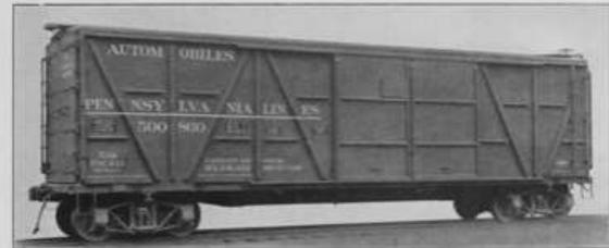
Fig. 43—Pressed Steel Frame 30-Ton Capacity Automobile Car. Weight, 45,100 lb. Inside Length, 40 ft. 5 in.; Inside Width, 9 ft. 10 in.; Double Height, 9 ft. 2 in. Pennsylvania Railroad.
