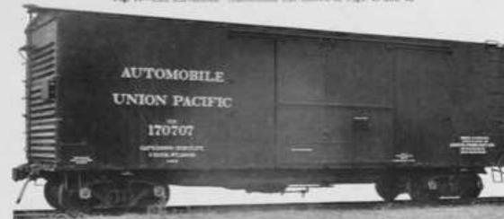
Fig. 45—Steel Frame 30-Ton Capacity Automobile Car. Weight, 46,400 lb. Inside Length, 40 ft. 4 in. Builder, Baltimore Steel Car Company. (See Fig. 44 and 46.)
