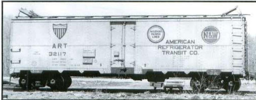
Originally a 1941 car in the 24200-24349 series, ART 32117 was renumbered in the early 1950s when equipped with electric air-circulating fans. Its shown here as repainted in the mid-1960s with placard boards lowered and all stenciling in black. Norfolk & Western heralds replaced the Wabash flags after the N&W acquired the Wabash in 1964. —Tom Martorano collection
