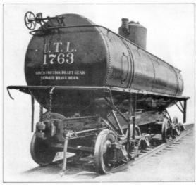
Fig. 89. Tank Car, Structural Steel Underframe. Capacity, 6,000 gals.
