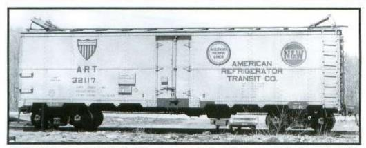
Originally a 1941 car in the 24200-24349 series, ART 32117 was renumbered in the early 1950s when equipped with electric air-circulating fans. Its shown here as repainted in the mid-1960s with placard boards lowered and all stenciling in black. Norfolk & Western heralds replaced the Wabash flags after the N&W acquired the Wabash in 1964. —Tom Martorano collection
