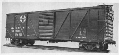
Fig. 30—Atchison, Topeka & Santa Fé 50-Ton Steel Frame Single Wood-Sheathed Box Car. Inside, Length 40 ft. 6 in., Width 9 ft. 2 in., He'ght 9 ft. 6¼ in., Capacity 3,550 cu. ft. Weight 48,700 lb. Builders, American Car & Foundry Company and General American Car Company.
