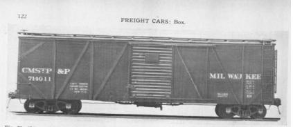
Fig. 28.—Chicago, Milwaukee, St. Paul & Pacific 50-Ton Single Wood-Sheathed Box Car. Inside, Length 40 ft. 6 in, Width 8 ft. 9 in., Height 9 ft. 3 in. Capacity 3,276 cu. ft. Weight, 46,300 lb., Load Limit, 122,700 lb. Builder, The Bettendorf Company.
