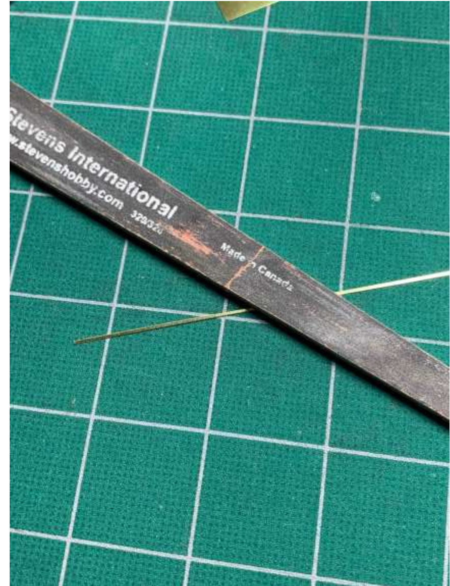
Using a sanding stick to smooth edges to remove slight raised edge
