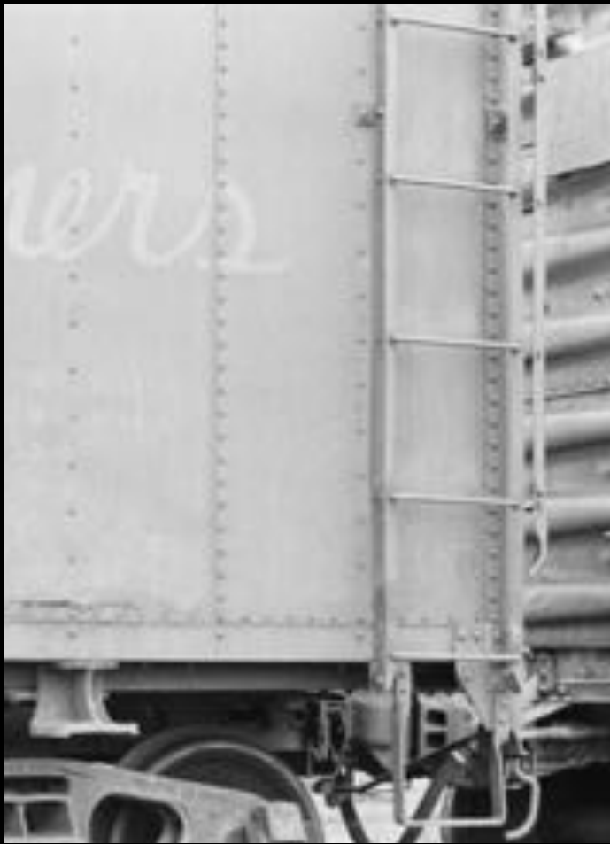
Combo 'Style' and sill step bracket
