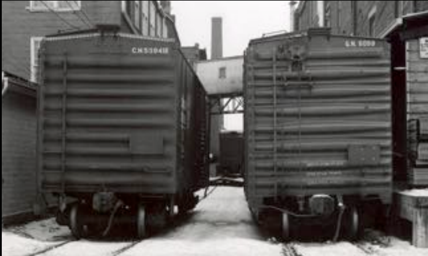
Typical Canadian and US Postwar Boxcar Ladder Configurations
