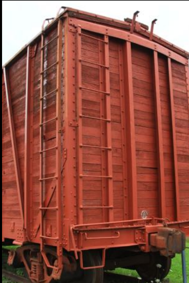
Right side of end rungs riveted to end brace
