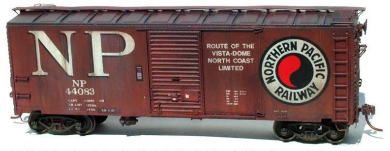
InterMountain undecorated model with rebuilt side sills, Westerfield door, Plano running boards, ModelFlex custom paint and lettered with Microscale decals. © C. Frissell
