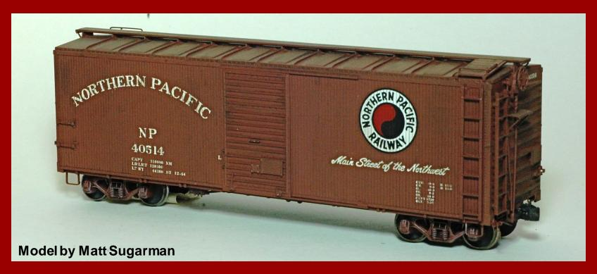
"40514 is a RC 10' AAR square corner post car w/ scratch-built sides from Evergreen, correct NP low track door and 7 rung ladders (I had a Sunshine kit of this car and was unhappy with it, so I scratch-built my own sides with Evergreen wood freight car siding and Archer rivet decals)"
