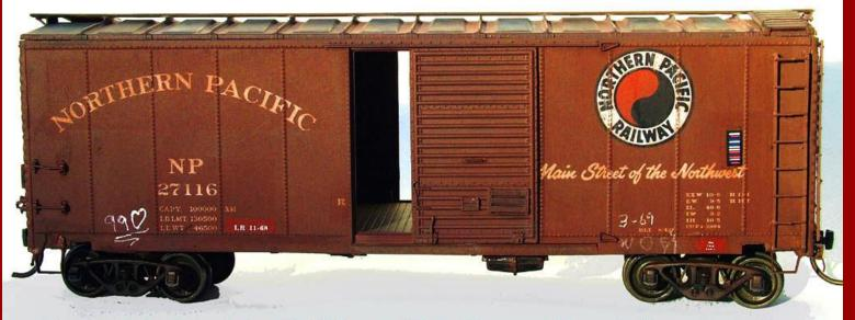
Intermountain decorated and built kit, retrofitted with correct 8-rung ladders, door guides, coupler lift bars, Kadee brake wheel, and Proto2000 trucks
