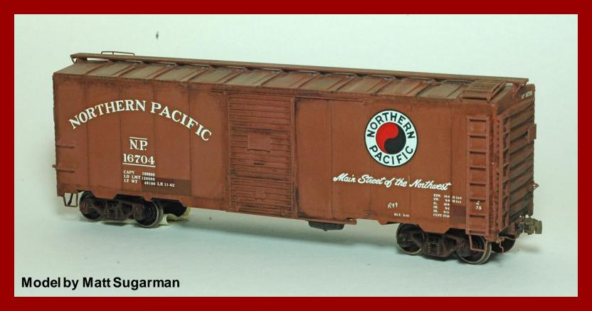
"16704 is a IMWX 10' AAR w/ tabbed sill, correct NP low mounted bottom track door and 8 rung ladders."
