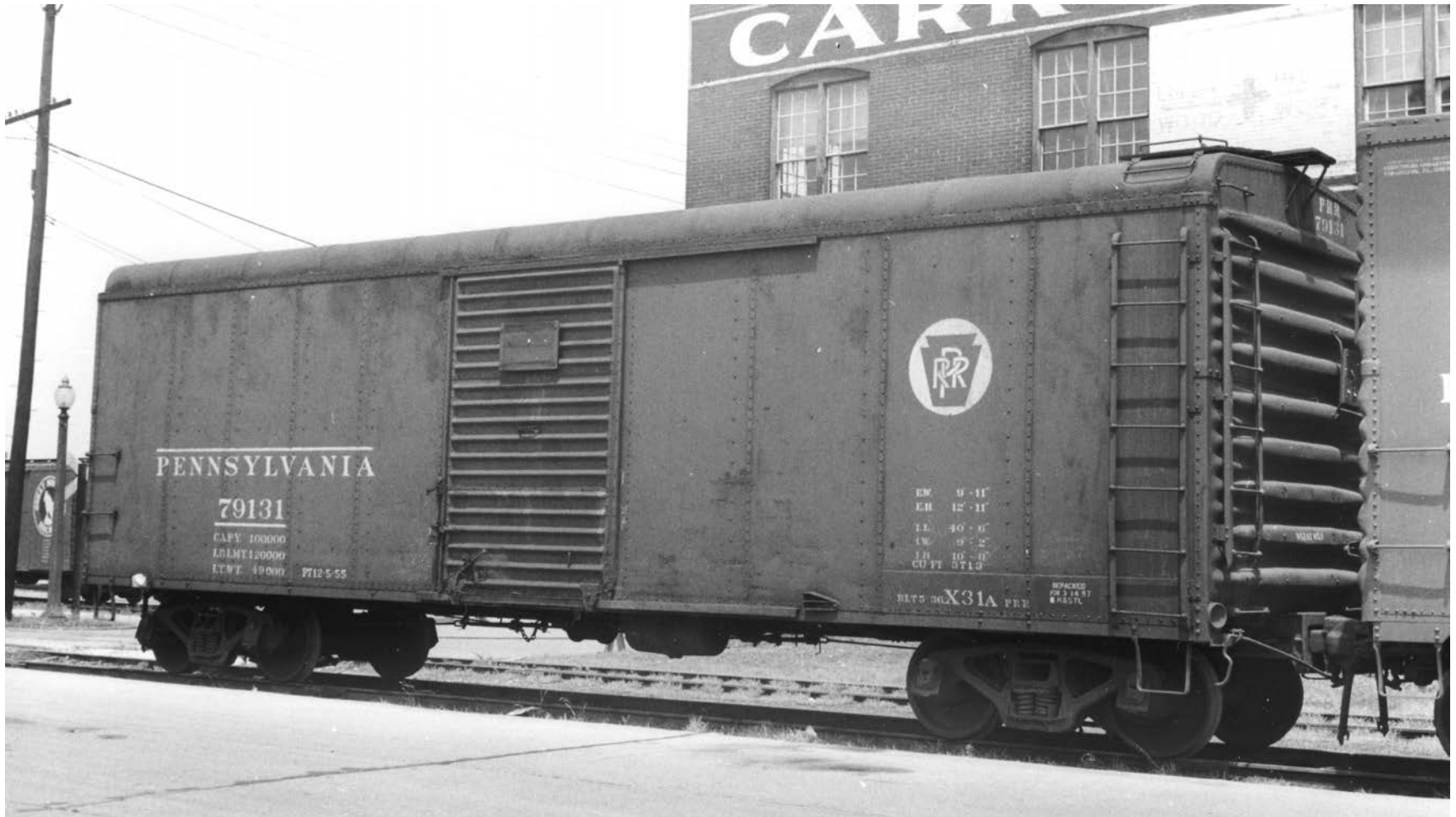
Reweighed 5-55, patch panels on two sheathing sections at A end, all-coil trucks, Joe Collias collection
