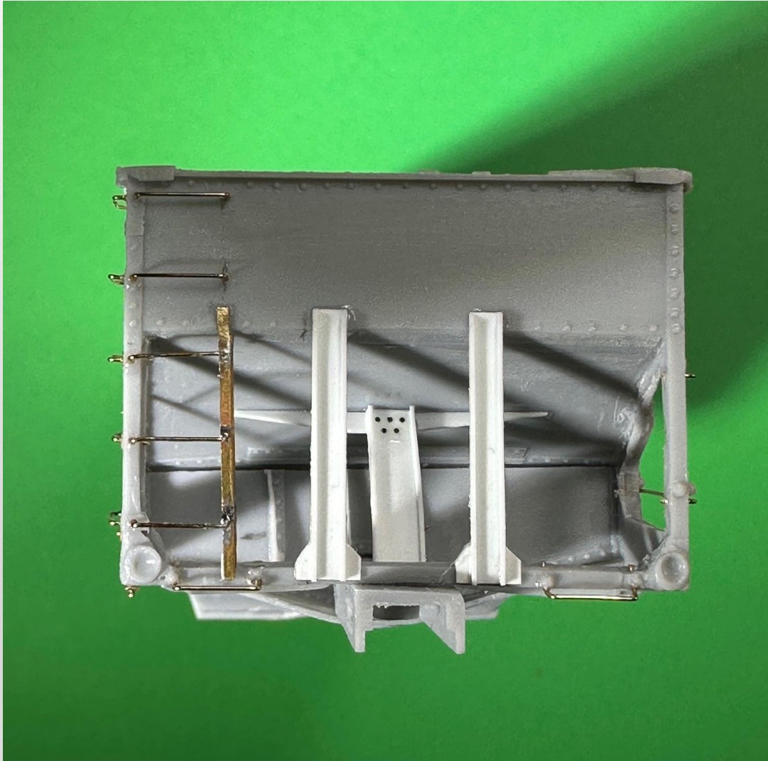
A End showing new end support brackets and slooe sheet brace
