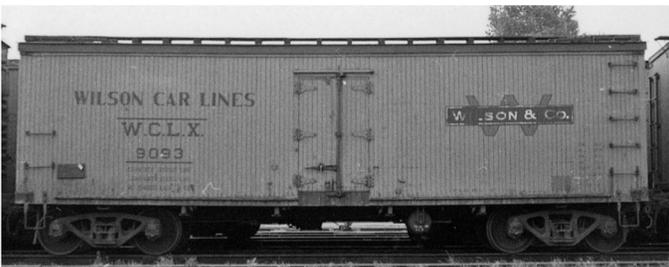
Medium W Scheme - Used circa 1947 - 1949 for repainted and new cars in WCLX 9201 – 9350 series. Estimated at 7' wide over center band.
