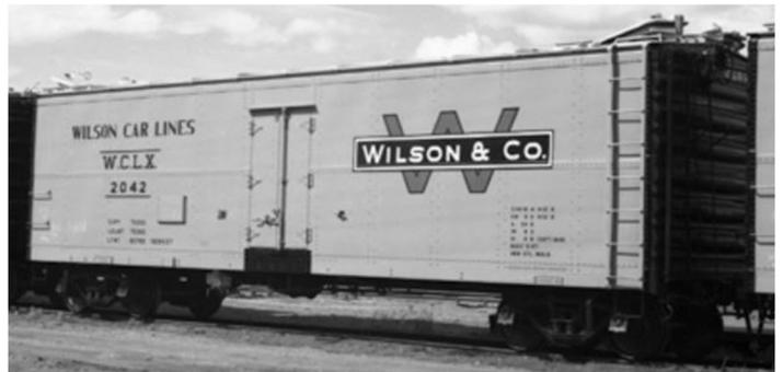
Large W Scheme - Used from 1952 on for both repainted and new cars including the last of the wood cars WCLX 9456 – 9605 as well as the PC&F steel cars in WCLX 2000 – 2799. Estimated at 10' over the center band.
