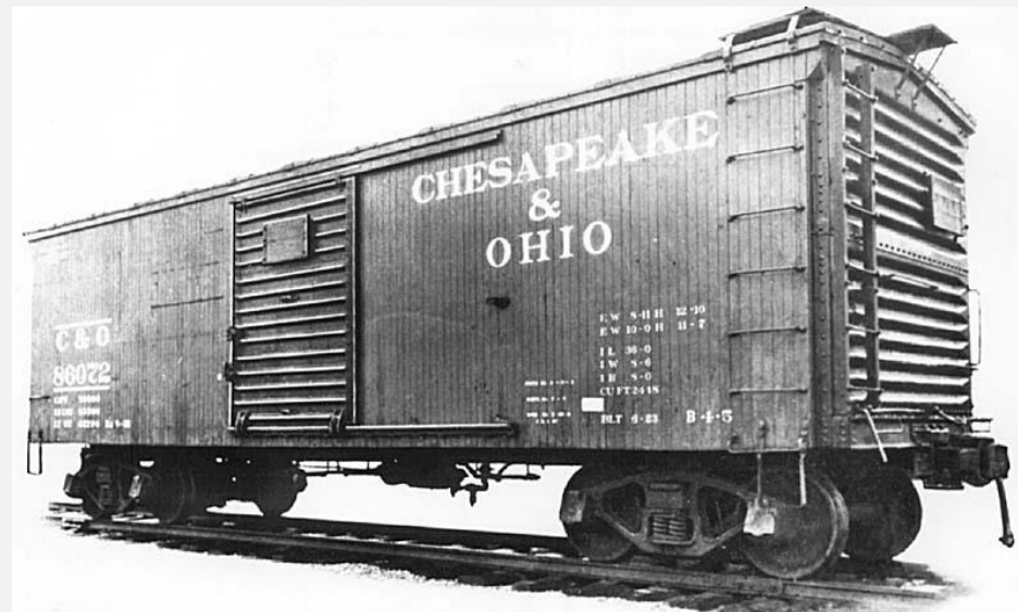
In 1924 the C&O bought three groups of "modern" short boxcars, and had rebuilt them in the late 1930s. The road still had 523 of them in 1950 but began retiring the remaining cars in bulk that year. By 1953 they were gone, except for a few in MOW service.
