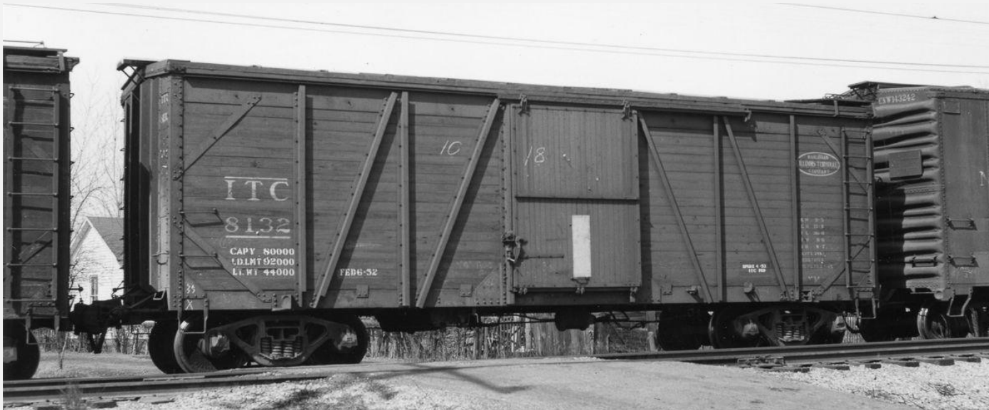
The Illinois Terminal had a small fleet of 38-foot single sheathed boxcars, and ran them past the end of electrification. In 1960 there were still 86 of them running in revenue service.
