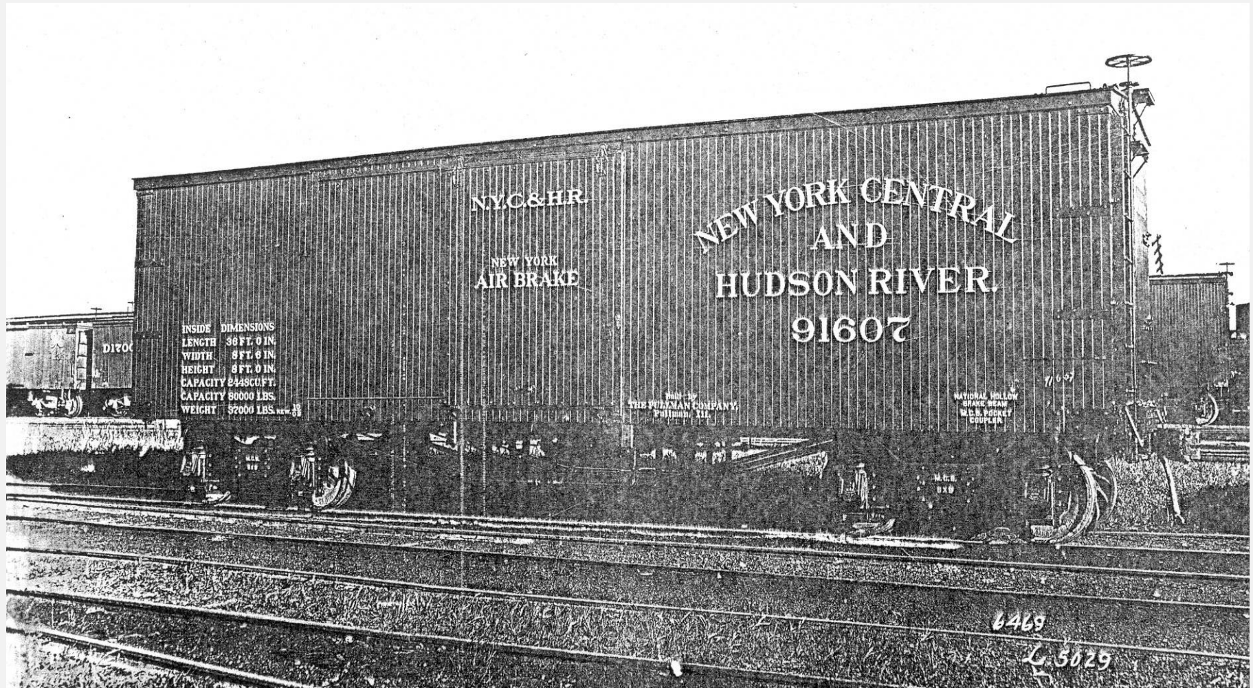
This NYC&HR boxcar, built by Pullman in 10/1902, perfectly adheres to the 1894 MCBA house car standards.
