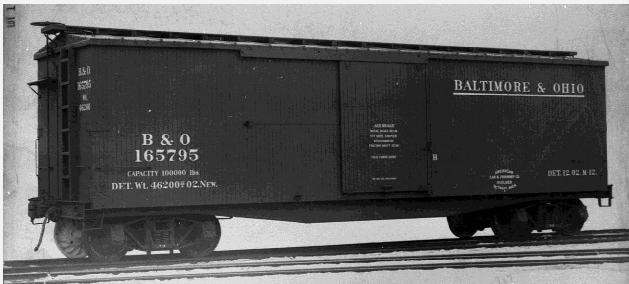
The B&O purged most of their short boxcars from the roster during the Depression, but a few stragglers remained after WWII, including a few examples of these 1902-built cars. Six clung on past 1957 but were gone by the end of 1959.
